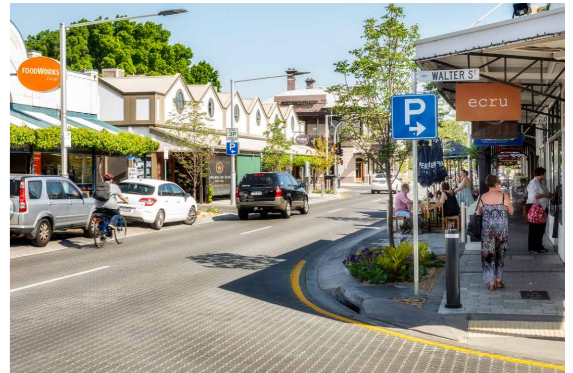
Narrowing corner radii at intersections helps to reduce vehicle speeds and pedestrian crossing distances.
